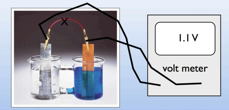
Mix up "standard" concentrations I M Zn<sup>2+</sup> and I M Cu<sup>2+</sup> (note this is very concentrated) Principles of Chemistry II
