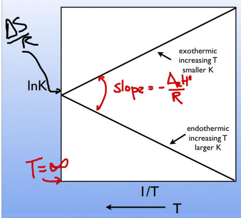
y = mx + b y is InK x is I/T  $m \text{ is -}\Delta_RH^\circ/R$  $b \text{ is }\Delta_RS^\circ/R$
