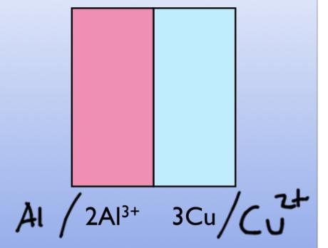
We can make use of these electrons moving between the two species if we can physically separate the two reactions
