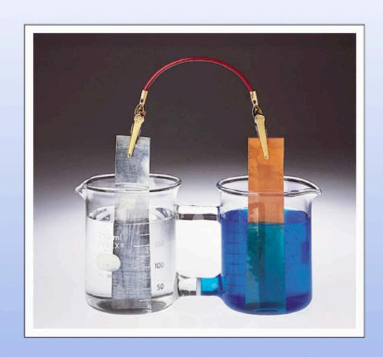
Salt bridge connect the circuits by allowing ions to flow between the two regions
