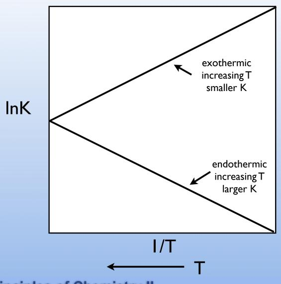
y = mx + b y is InK x is I/T  $m \text{ is } -\Delta_R H^\circ/R$  $b \text{ is } \Delta_R S^\circ/R$
