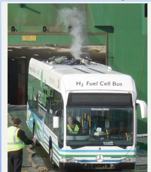
In the photograph above the first bus is unloaded from the ship, with the pure steam rising from its exhaust pipe visible at the rear.
