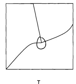
The picture at left shows a possible phase diagram for a pure substance around its solid, liquid, vapor triple point. Based on the slopes and curvatures of the lines, it is possible that this a diagram for an actual substance? Why or why not?
